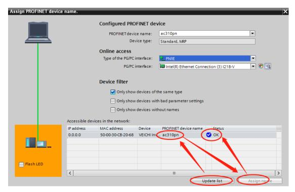
If there are more than one other devices, you can select other devices to assign the name. After receiving the assigned name, the slave station will save the name. The master station distinguishes each slave station by the device name. The essence of assigning the name is to bind the device name and MAC address. After modifying the name of the station device in the configuration, the name must be reassigned
