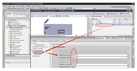
Switch back to the network view. If you need to add more slaves, repeat the above. If the configuration is the same, you can copy the slave directly, and then modify the IP address and device name
