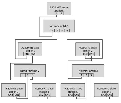
Figure 3.3. Schematic diagram of connection tree
