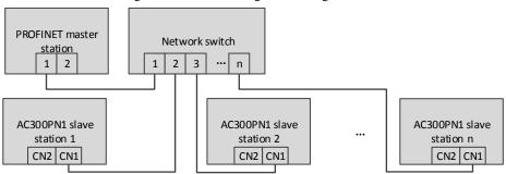
Figure 3.2 Schematic diagram of star connection
