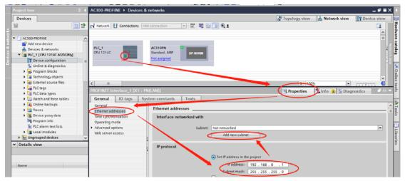
Click "unassigned" of AC310PN, and click "PLC\_1. PROFINET interface\_1"
