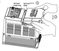
Dismantlement: At the tail of the frequency inverter, there is a special dismantlement hole design. Put your fingers into the hole, upwardly pull the cover with a little force until the buckle between the tail-hood and the crust tear off, and then removed tail-hood down.
